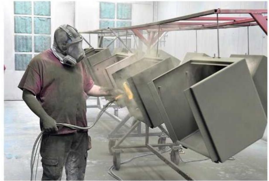
Jake P. Sukalski powder coats a rack of metal boxes at D&K Powder Coating.
